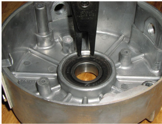
Figure 16-11 Bearing Retaining Ring
