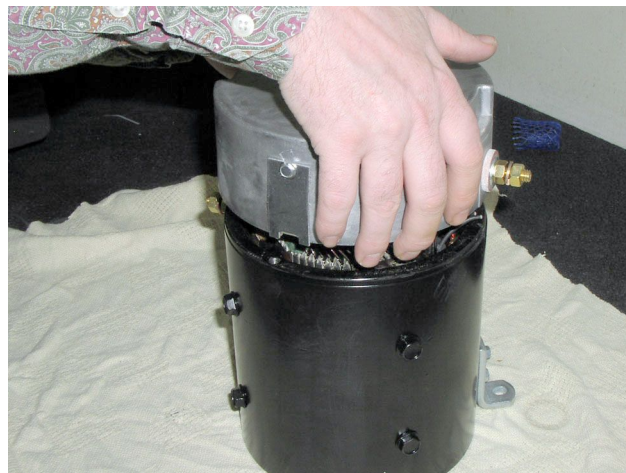
Figure 16-7 End Cap Removal
