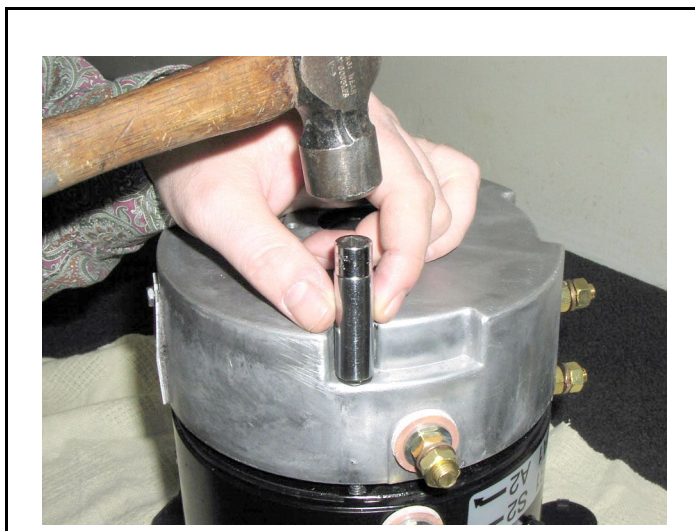
Figure 16-6 End Cap Disengagement
